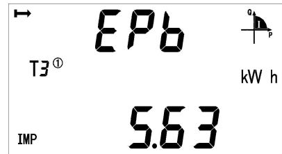
Current forward active energy on B phase
