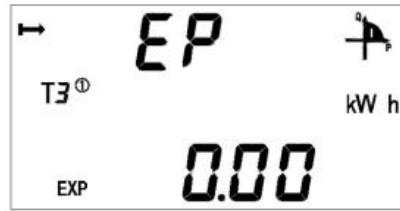
Current reversing active total energy
